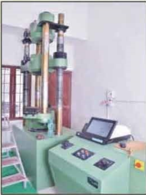
Computerised Universal Testing Machine (Capacity 1000 kN)
