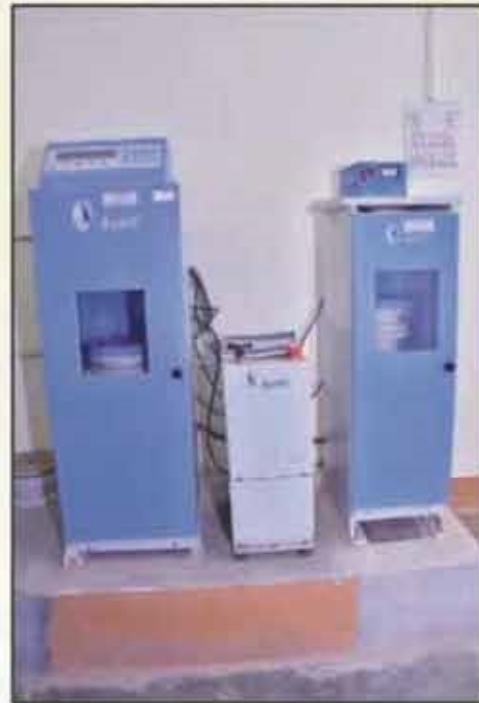
Computerised Compression Testing Machine with controlled stress rate (Capacity 2000 kN & 500 kN)
